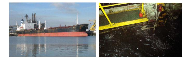
On 6<sup>th</sup> March 2014 with the vessel afloat at Lagos outer anchorage, a huge quantity of water entered from the sea chest and caused the immediate, heavy flooding of the engine room with severe damages to vessel's machinery.
